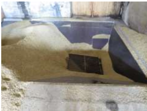
Figure 31. Intake of grain to the dryer.
