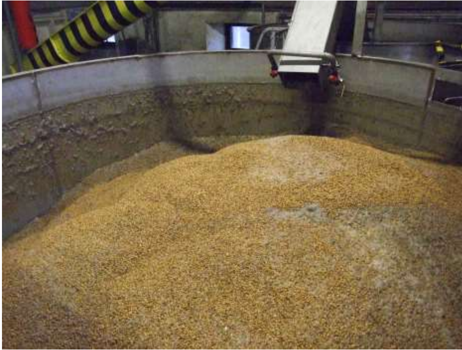
Photo 3. Grain after draining following the third step.
