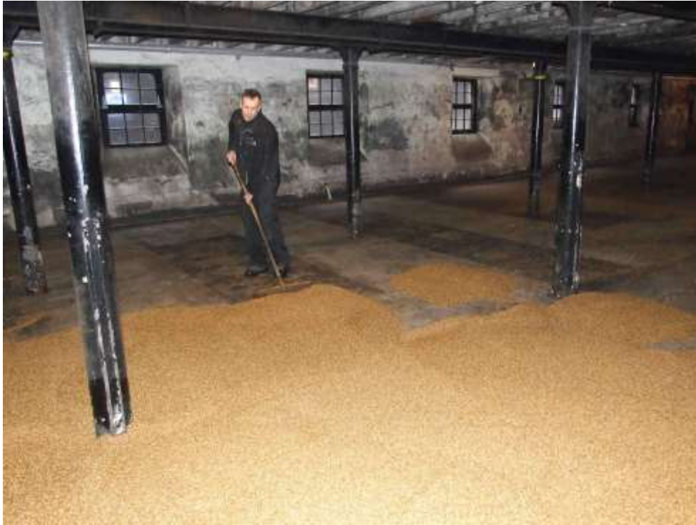
Photo 7. Spreading out the grain on the malting floor.
