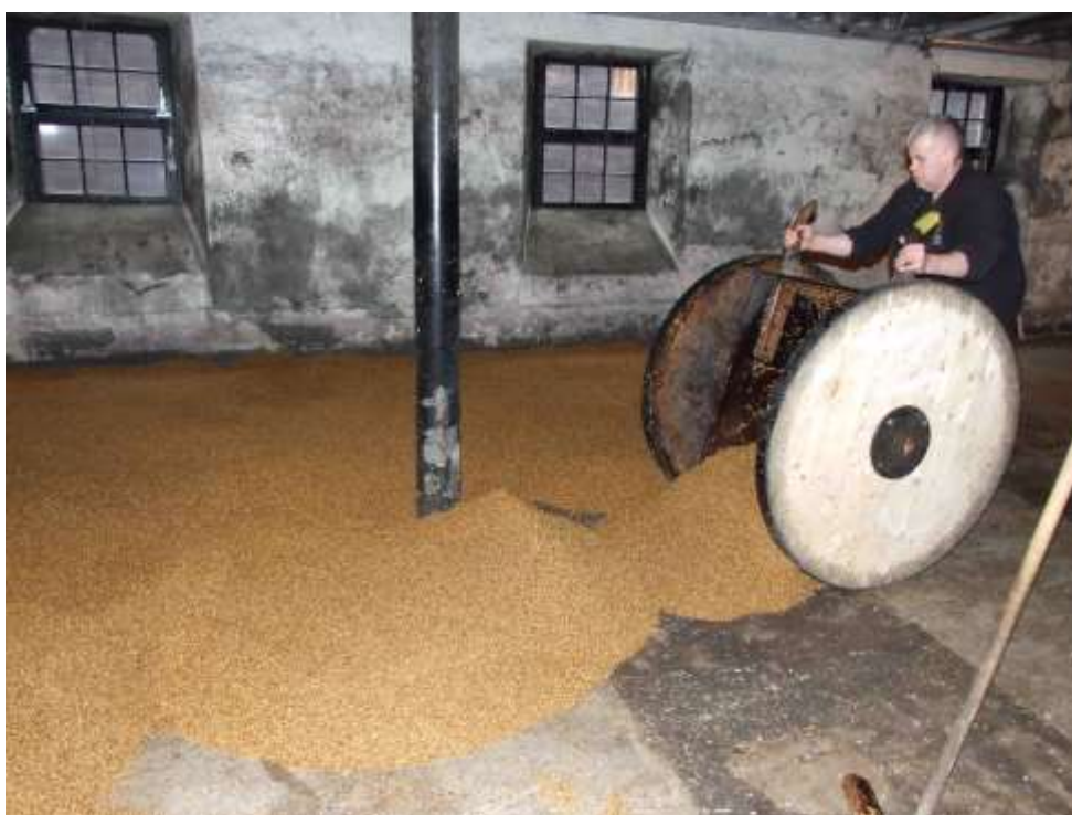
Photo 6. Casting steeped grain on the malting floor.
