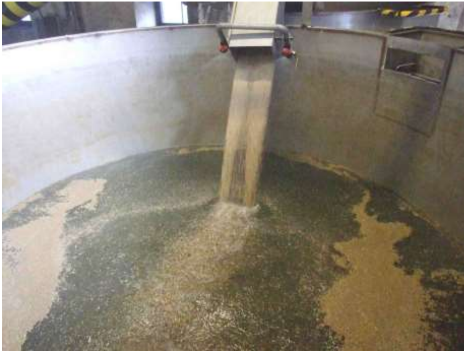
Photo 1. Transferring grain into the steeping vessel.
