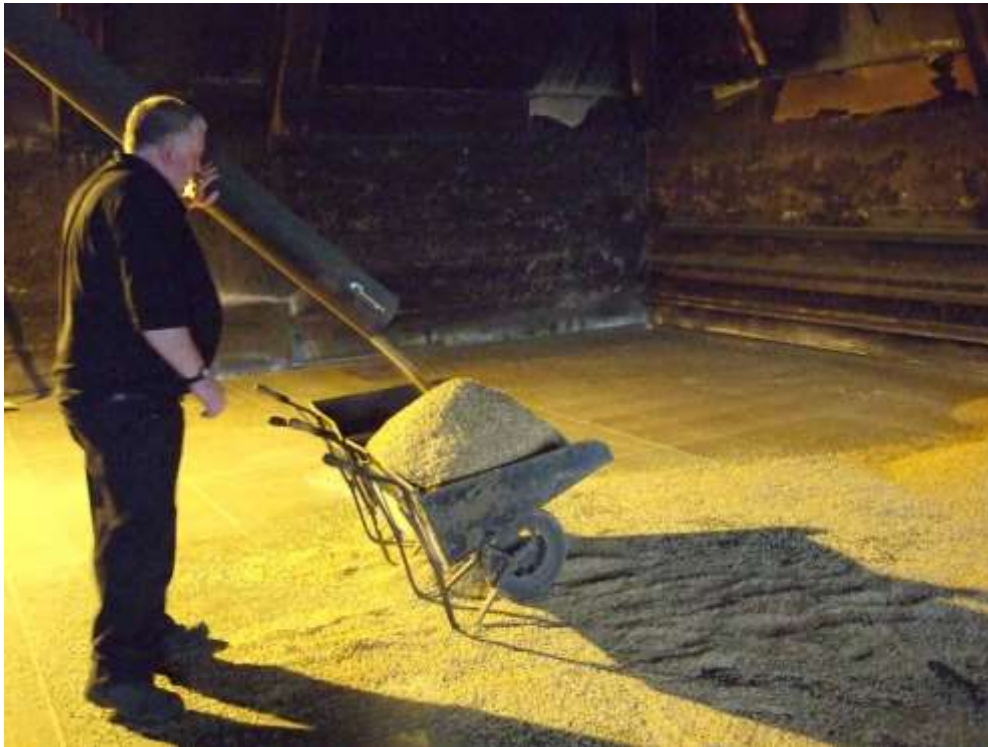
Photo 13. Spreading the green malt on the kiln floor.
