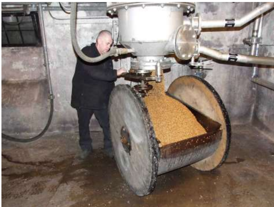
Photo 5. Unloading grain from the steeping vessel.
