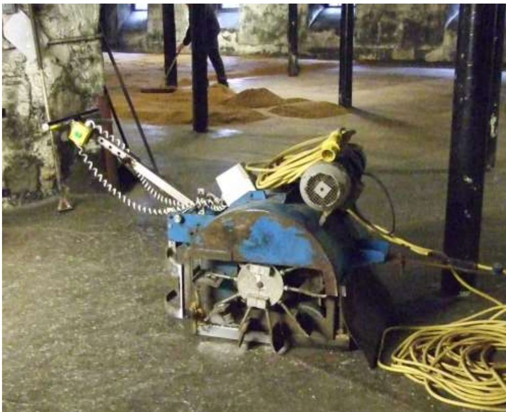
Photo 8. Machine used for turning malt
