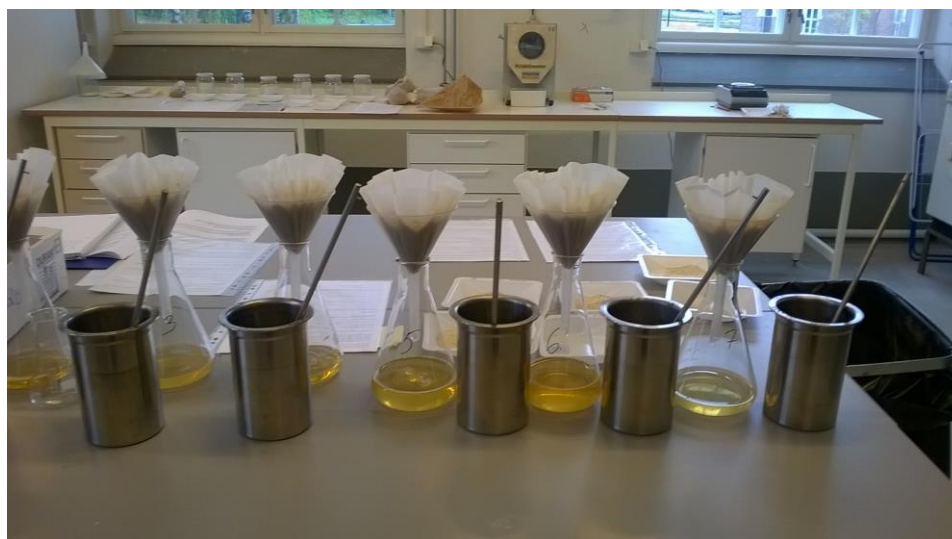
Fig. 5. Mash of the 7 barley varieties being tested for filtration rate.
