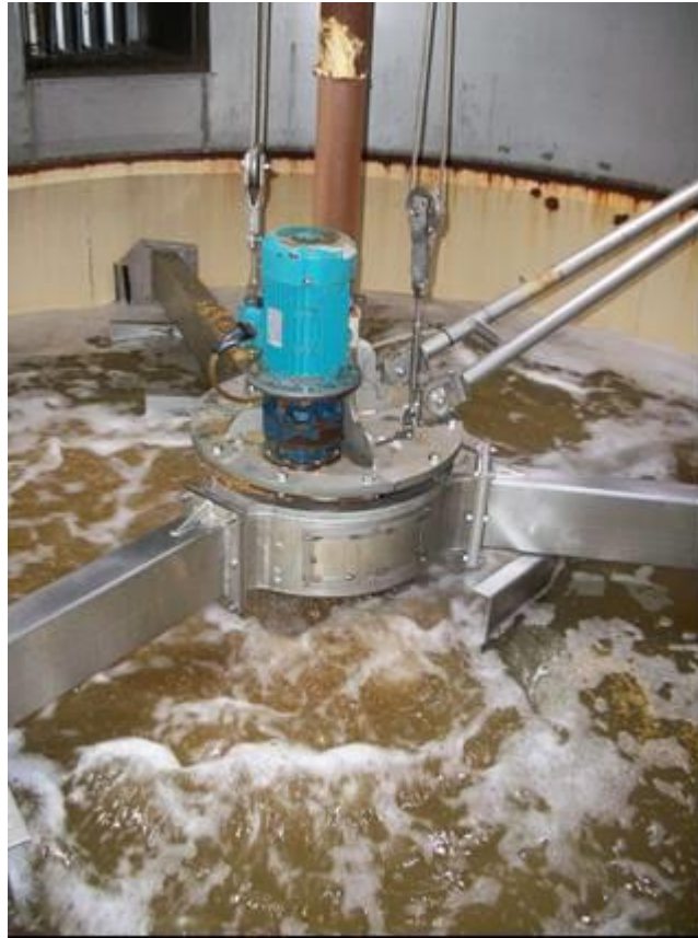
Fig. 3. Bere being steeped in the Pilot Vat at Crisp Malt, Great Ryburgh.
