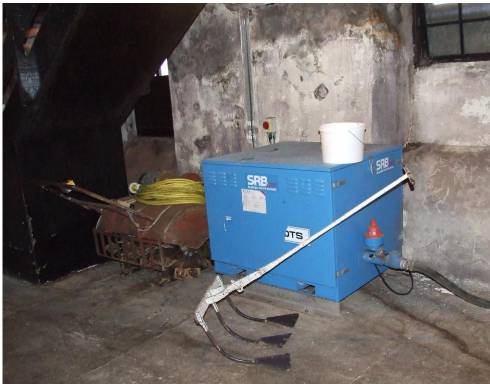
Photo 9. Manual rake used for ploughing the malt.
