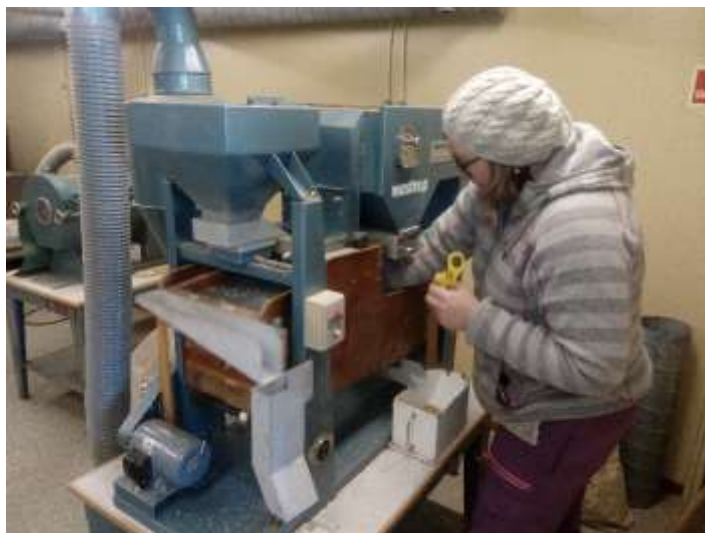
Fig 16. After the malting ended, we received a new screen to our small-scale seed grading machine from Westrup. This is a screen with 2,5 mm slotted holes, meaning for the future we can sort out the larger grains for malting.
