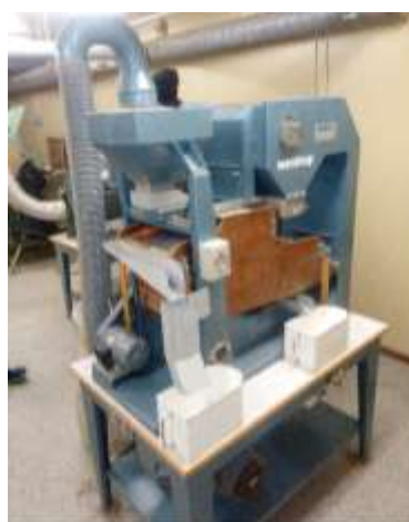
Figure 4 and 5. Small scale grain cleaner and grain sorter from Westrup, from Nibio Holt, Norway.
