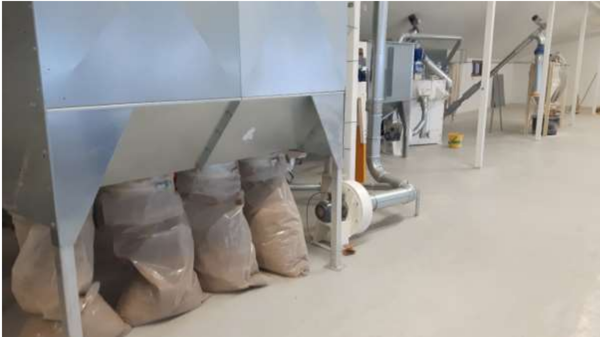
Figure 16. Dyrk Mølle from Norway chose to buy a complete milling line from the company Engsko in Denmark. The mill they chose has a capacity of 200 kilos per hour. The complete line was installed in the fall of 2017.
